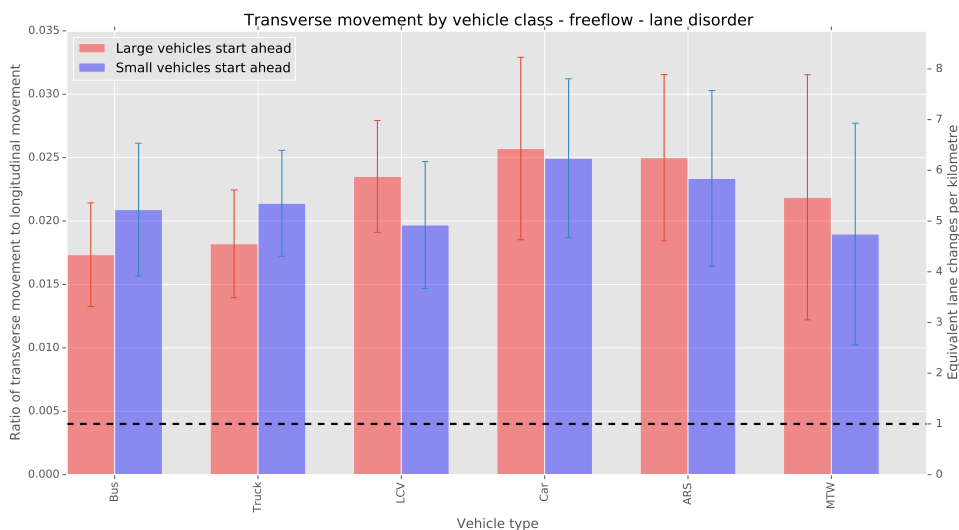
FIGURE 4.7: The degree of weaving (ratio of transverse to longitudinal movement) for each vehicle class in freeflow simulations of 20 agents distributed according to Table 4.3, on a 3-lane road of width 12m and length 150m with periodic boundaries. Each value is the average of 50 simulations, with error bars indicating the standard deviation between all vehicles aggregated within each class, aggregated from separate simulation runs. To eliminate transient effects from starting conditions, the first 15% of each simulation is discarded. The right-hand vertical axis is a rescaling of the primary axis in units of lane changes per kilometre, based on a lane width of 4m. The horizontal broken line indicates an approximate typical number of lane changes per kilometre for urban developed-world traffic [41].
