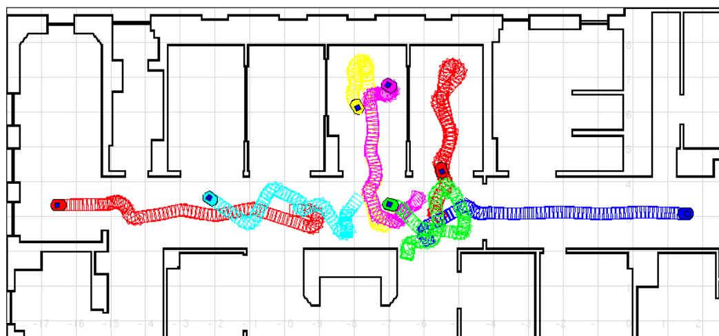
Figure 4.1: A typical Player/Stage simulation, showing a number of variously-coloured robotic agents traversing a 2D map. Reproduced from [26].
